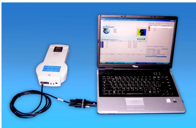
Fig 2: Portable module connected to USB Port for log transfer
